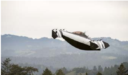
Opener's single-seat eVTOL BlackFly can fly 25 miles at 62 mph. (Source: Opener)
