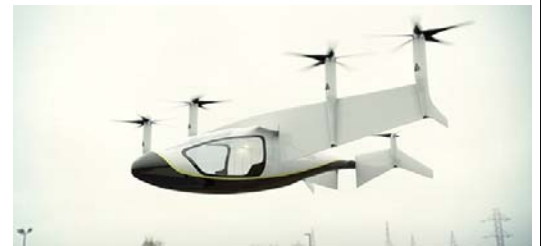
The concept uses gas turbine technology to power an electric battery and the wings are able to rotate 90 degrees. As well as a taxi, the vehicle could also be deployed for personal, cargo and military use, said Rolls-Royce: The forward wing rotates 90 degrees to enable vertical takeoff and landing. (Source: Rolls-Royce)
